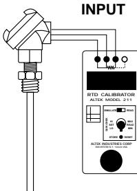
Whenever READ mode is selected the word READ will appear on the LCD. The Model 211 can measure temperatures in two ranges with resolution of 0.1 $^{\circ}$  and 1 $^{\circ}$ . The display is updated twice per second to continuously track fast moving temperatures. Using three or 4-Wire hookups provides accurate readings in long cable runs.
